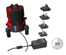
Charge the Li-Ion battery before using it for the first time. While charging, the instrument may heat up. This is normal and should not affect the instrument's lifespan or performance. At the recommended storage temperature of -20°C to +30°C (-4°F to +86°F), batteries containing a 50% to 100% charge can be stored up to 1 year. After this storage period the batteries must be recharged.
