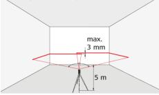
Place the lock switch in the "Unlocked" position. Position the instrument approx. 5 m away from the wall. Direct the instrument at the wall and switch on. Activate the laser line and mark the intersection point of laser crosshairs on the wall. Swivel the instrument to the right and then to the left. Observe the vertical deviation of the horizontal line from the marking. If the difference does not exceed 3 mm, then the Leica Lino L4P1 is within tolerance.
