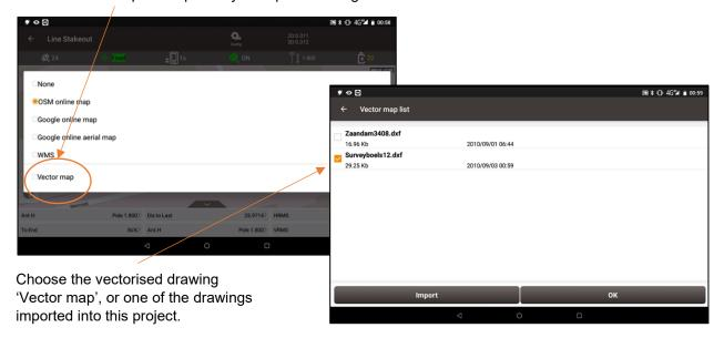
In the drawing, select the line/arc you want to stake out by clicking in the centre of the line element. It is also possible to stake out points in this menu.
