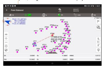
When the position of the point to be staked out is approached to a few centimetres, the screen changes as shown below. The tilt position of the GPS pole is also visible graphically.
