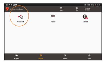
Search for the antenna via Bluetooth; the serial number can be read at the bottom of the antenna
